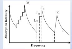
The spectrum show sharp discontinuity in the absorption spectrum of a substance.
