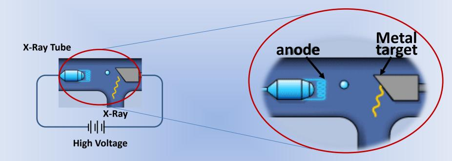
X-rays are produced by accelerating electrons with a high voltage and allowing them to collide with a metal target.
