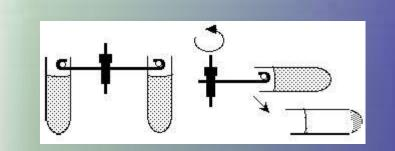
Longer distance of travel may allow better separation, such as in density gradient centrifugation. Easier to withdraw supernatant without disturbing pellet.
