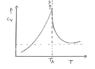
For T>TX the behaviour of liquid He & normal and it colled He I and for T<T, liquid He shows remarkable properties such as zero viscosilty or superfluidity, zero entropy so liquid He is called He II.
